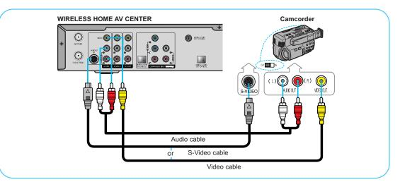
Connect a Video/Audio cable between the VIDEO or S-VIDEO / L - AUDIO - R jacks to the WIRELESS HOME AV CENTER and the VIDEO or S-VIDEO / AUDIO output jacks on the camcorder. (Note: For better video, use an S-VIDEO cable.)
